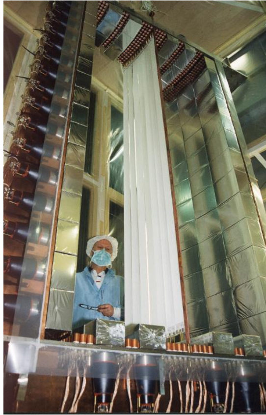
Figure 4 - The commissioning of a sector of the NEMO-3 detector including source strips without tracking Geiger cells.
